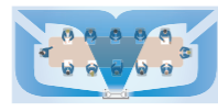
The airflow is optimally controlled to provide improved comfort in a narrow room.
